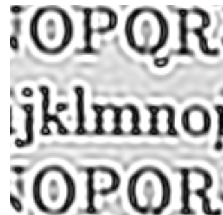
(c) Restored by Gaussian PSF Model
