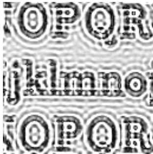
(b) Restored by Geometric PSF Model
