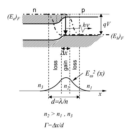
Forward biased p-n homojunction  $\Delta x$  – region of light amplification (G > 0)
