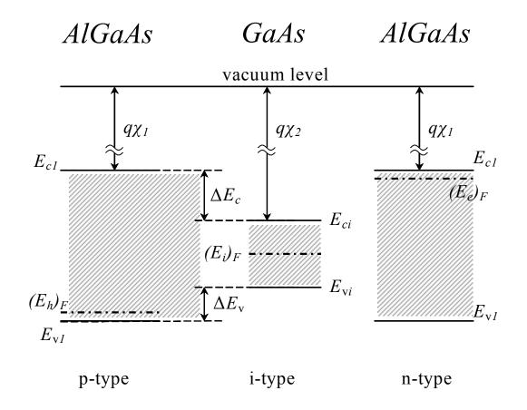
p-i-n heterojunction Band discontinuities and band bending at equilibrium (V = 0).
