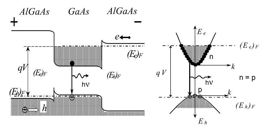
Forward biased p-i-n double heterostructure (DH). Emission of photon. There is population inversion in the narrow gap semiconductor of DH, i.e.  $f_{\rm e}+f_{\rm h}>1$
