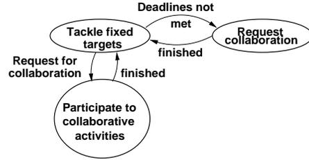
**Figure 3. Decentralized controller for UAV operation**
