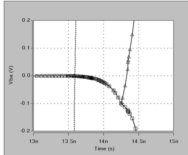
Fig. 7. Transients in the latch phase:  $\square$ —no SEE hit;  $\triangle$ —SEE hit occurring within its critical time.
