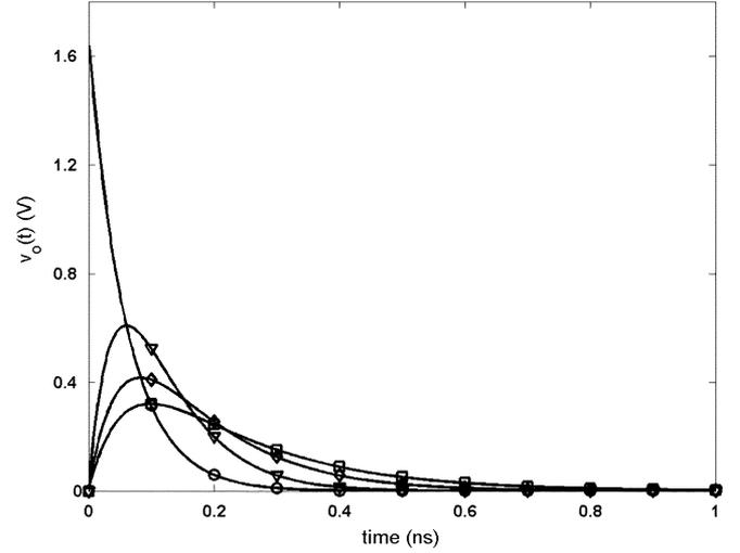
Fig. 3. Voltage transient in (4):  $\circ - \tau = 0$ ;  $\nabla - \tau = 60$  ps;  $\diamond - \tau = 120$  ps;  $\square - \tau = 180$  ps.
