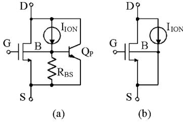
Fig. 5. (a) SOI MOSFET SEE model in [10] and (b) simplified model.
