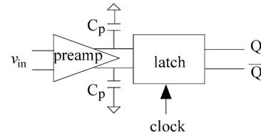
Fig. 1. Simplified structure of a latched comparator.
