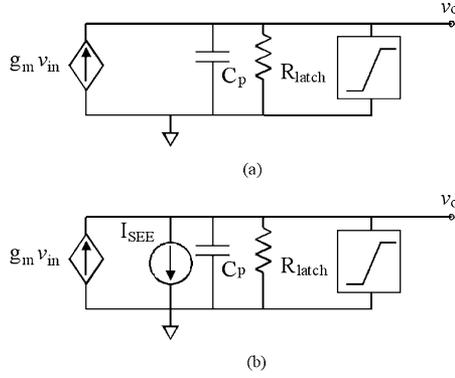
Fig. 2. Equivalent single-ended model for a latched comparator: (a) radiation-free environment; (b) affected by SEE.
