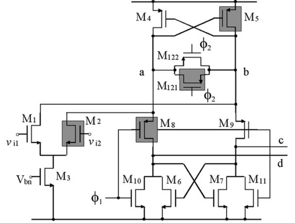
Fig. 4. Schematic of the simulated comparator.
