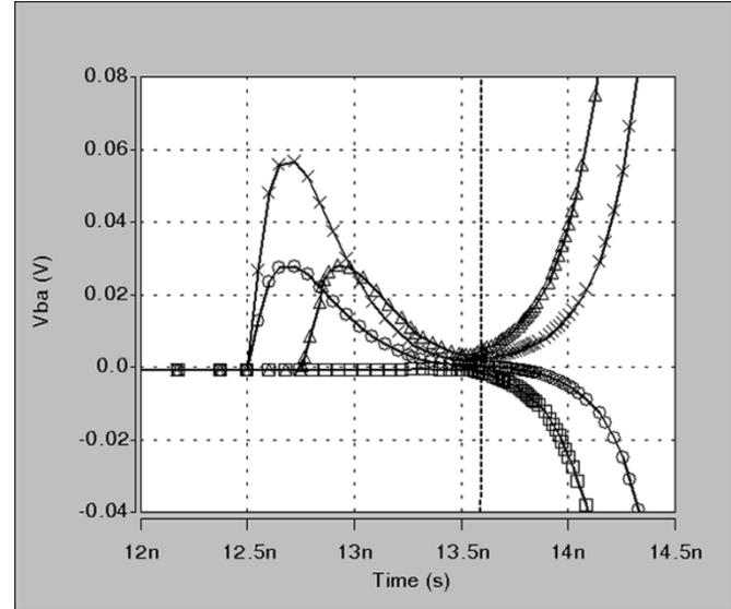
Fig. 6. Transients in the regeneration phase:  $\square$ —no SEE hit;  $\triangle$ —small amplitude hit occurring within its critical time;  $\circ$ —small amplitude hit occurring beyond its critical time;  $\times$ —large amplitude hit occurring within its critical time.
