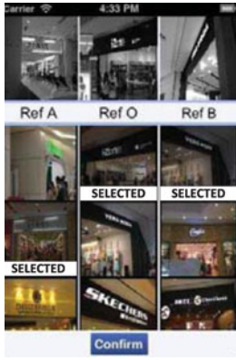
Fig. 17. The UI presented to the user for correction of image matching results. The top row are the three test images taken by the user, below each are the top 3 matched reference objects. The user can denote the correct match by tapping the thumbnail images.
