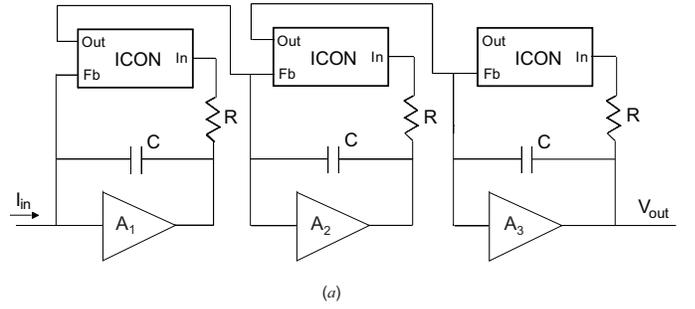
Fig. 8. (a) Implementation of the pulse shaper. (b) Schematic of ICON cell.
