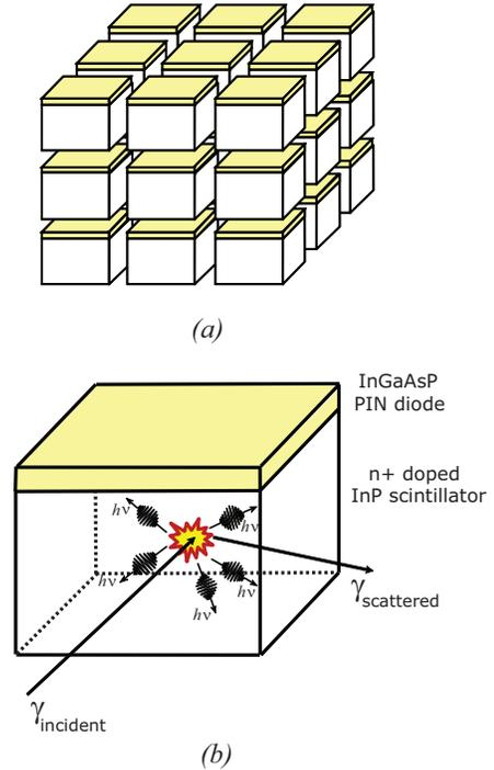
Fig. 1. (a) Illustration of a 3D scintillator array. Each unit contains the semiconductor scintillator as radiation detector and readout ASIC. (b) Semiconductor scintillator comprising a scintillator body and an integrated photodiode (top plate) on its surface. Since the thickness of the photodiode is a small fraction of the thickness of the scintillator body, we expect a negligible number of events to be generated in the diode.
