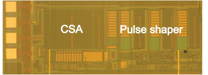
Fig. 9. Microphoto of the implemented single preamplifier channel, containing CSA and pulse shaper, in  $0.5 \mu\text{m}$  CMOS technology.
