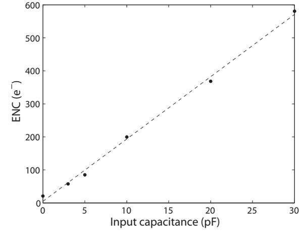
Fig. 13. Measured ENC as a function of the input capacitance.
