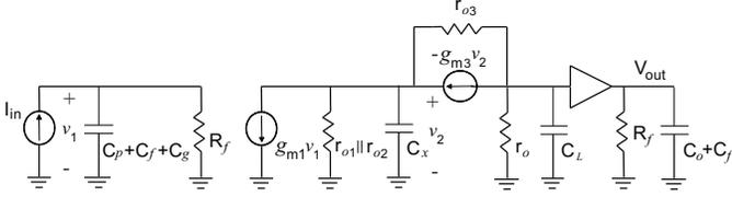
Fig. 7. Open circuit schematic of the first-stage voltage amplifier after breaking the loop.
