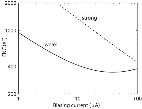
Fig. 2. Minimum ENC as a function of fixed biasing current, with no constraints on  $\tau$  and  $C_g$ . The input transistor is assumed to be either in the strong-inversion or in the weak-inversion regime.
