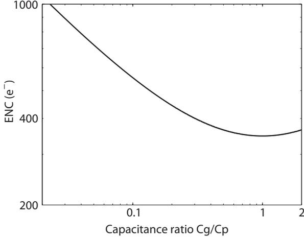
Fig. 3. Minimum ENC for a fixed capacitive ratio of  $C_g$  and  $C_p$ , with no constraints on  $\tau$  and  $I$ , when the input transistor is in the weak-inversion regime.
