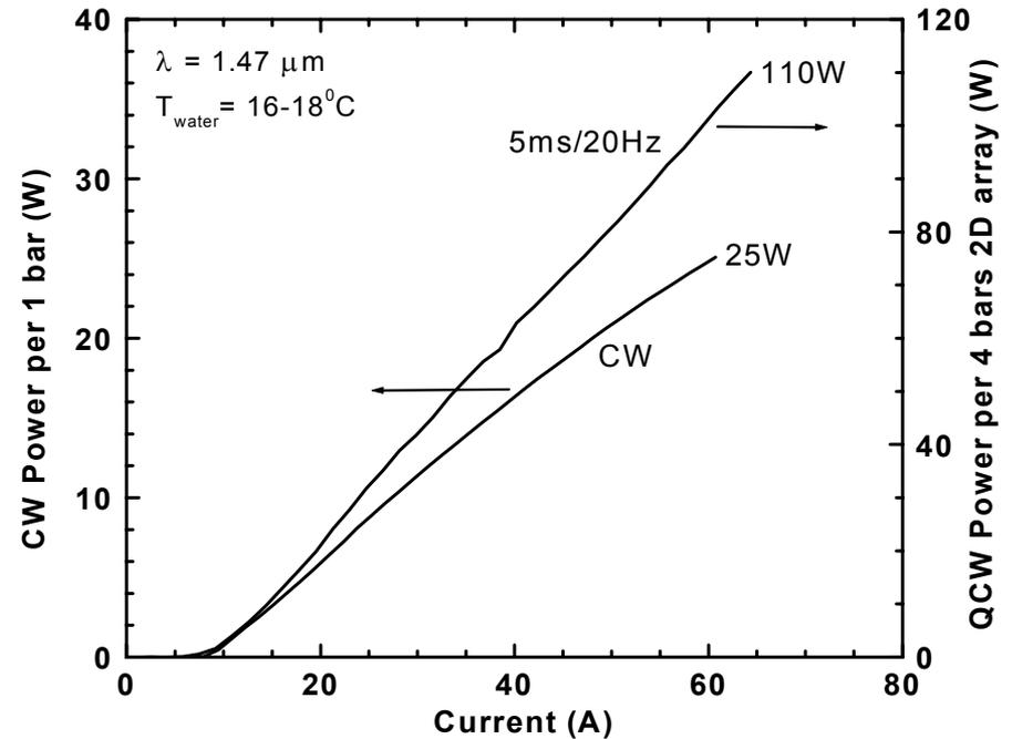
Performance of 1D and 2D 1.47 $\mu\text{m}$  laser diode arrays. Array were packaged into microchannel cooled heatsink and operate at CW and QCW conditions.
