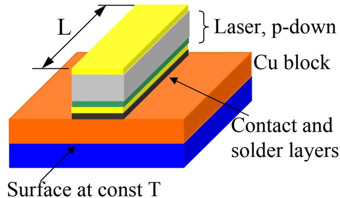
$$R_{\text{TH}} \propto \frac{1}{\text{cavity length, } L}$$
