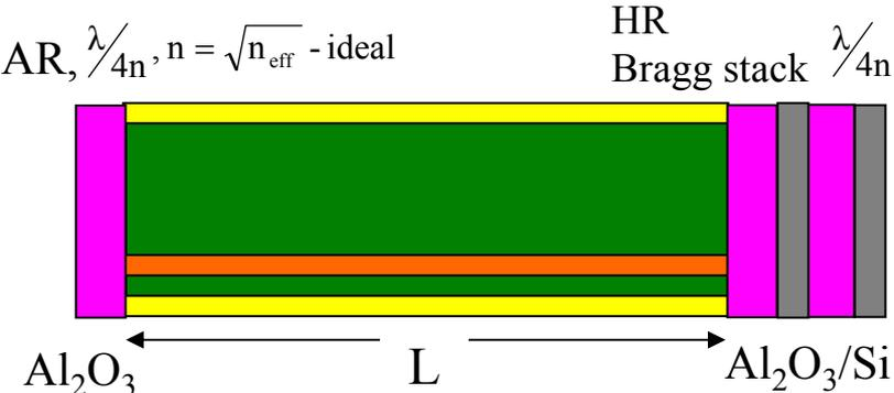
High power lasers are usually AR/HR (3-5%/95%) coated to direct all power to one mirror. The higher is the output power, the lower absorption coefficient the mirror coatings should have. Development of extra-low absorption optical coatings is now very important research direction due to numerous applications in solid state and semiconductor lasers industries.
