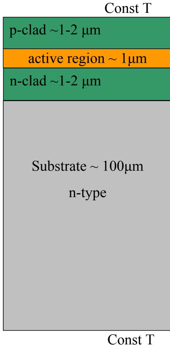
To eliminate the substrate thermal resistance we have to mount laser p-side down.
