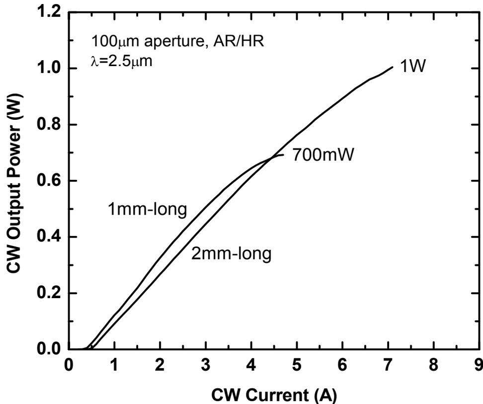
CW performance of high power lasers with broadened waveguide and low internal loss  $< 4\text{cm}^{-1}$ . Devices were In soldered p-side down on water cooled Cu blocks. Water temperature  $\sim 15^\circ\text{C}$ .
