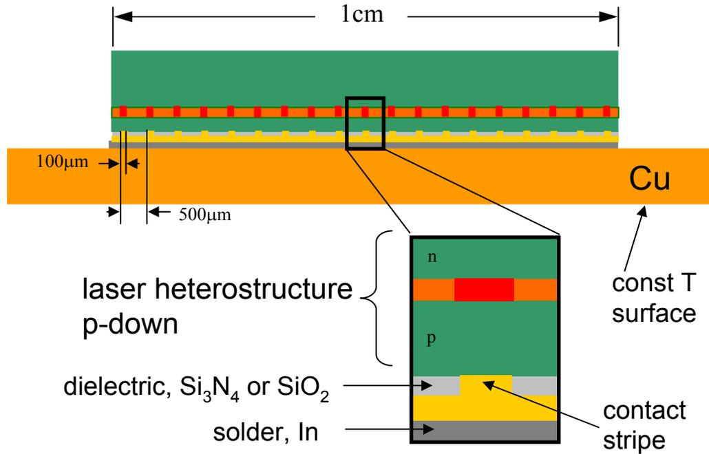
1D laser array is laser bar with emitters defined by metal contact stripes.
