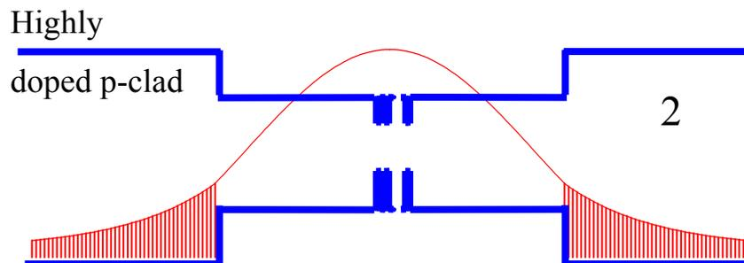
The efficiency of the broadened waveguide lasers are less sensitive to cavity length increase and long cavity lasers can be used for high power applications.
