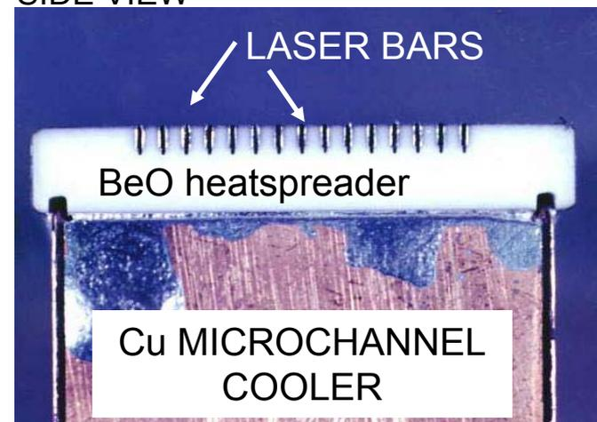
2D laser arrays can produce hundreds watt of CW output power. 2D arrays can be further combined into stacks of array and produce total power of  $>10kW$  in relatively compact package.
