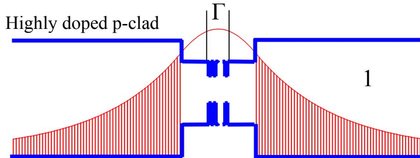
Confinement factor  $\Gamma$  for broadened waveguide devices is slightly reduced but the losses decrease dramatically resulting in net decrease of the threshold current density.
