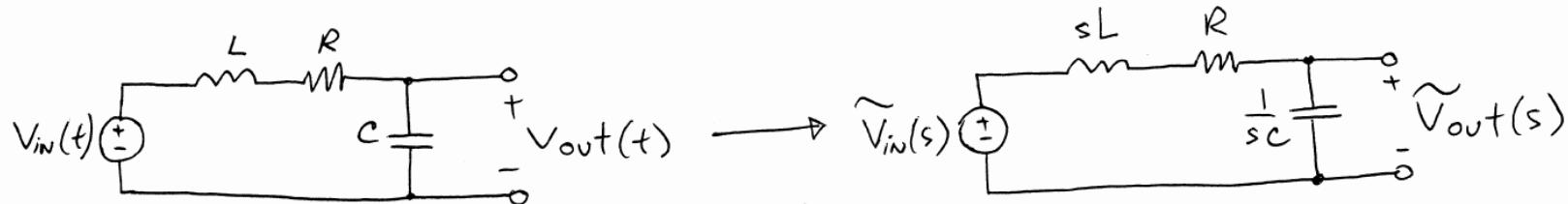
$$T(s) = \left| \frac{\tilde{V}_{out}(s)}{\tilde{V}_{in}(s)} \right|_{\substack{\text{ZERO} \\ 1C}} = \frac{\frac{1}{sC}}{sL + R + \frac{1}{sC}} = \frac{1}{LC} \cdot \frac{1}{s^2 + s \cdot \frac{R}{L} + \frac{1}{LC}}$$
