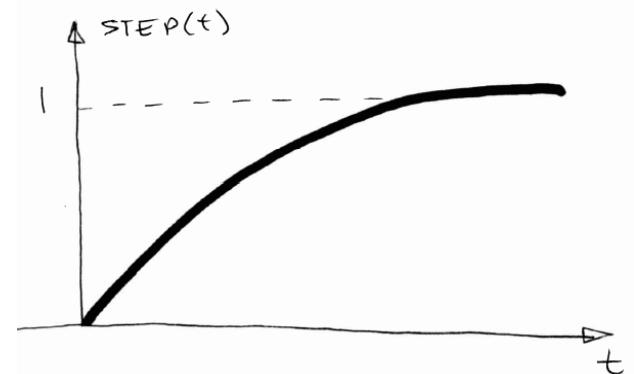
**Overdamped case – the circuit demonstrates relatively slow transient response.**
