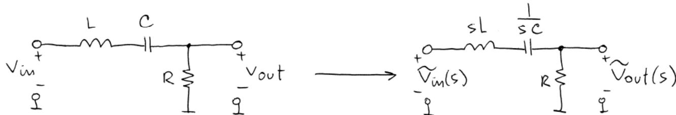
$$T(s) = \left. \frac{\tilde{V}_{out}(s)}{\tilde{V}_{in}(s)} \right|_{\text{ZERO } IC} = \frac{R}{sL + \frac{1}{sC} + R} = \frac{R}{L} \cdot \frac{s}{s^2 + \frac{R}{L} \cdot s + \frac{1}{LC}}$$
