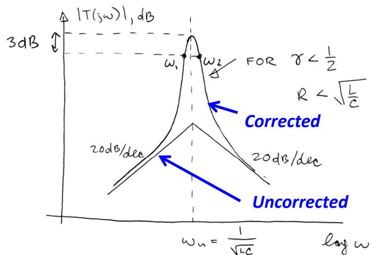
**Half power bandwidth:**  $|T(j\omega)|_{\omega=\omega_1 \text{ or } \omega_2} = \frac{1}{\sqrt{2}}$
