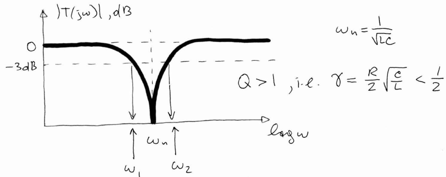
$$\text{BW} = \omega_2 - \omega_1 = R/L \quad ; \quad Q = \frac{\omega_n}{\text{BW}}$$
