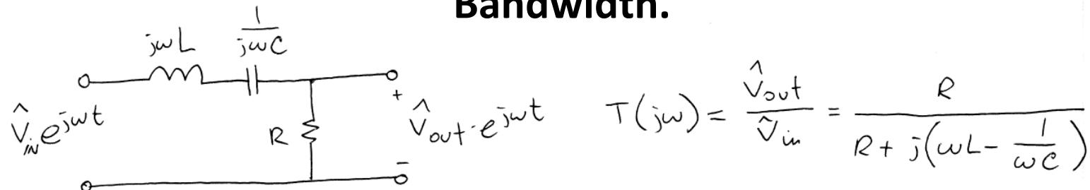
$$|T(j\omega)| = \frac{R}{\sqrt{R^2 + (\omega L - \frac{1}{\omega C})^2}} ; |T(j\omega_n)| = 1 ; \omega_n = \frac{1}{\sqrt{LC}}$$
