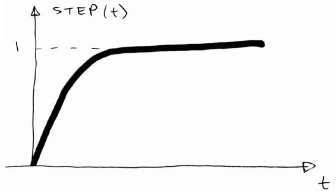
$$\text{step}(t) = L^{-1} \left[ \frac{T(s)}{s} \right] = \frac{1}{LC} L^{-1} \left[ \frac{1}{s(s-p)^2} \right]$$
