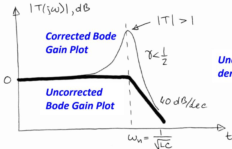
Underdamped case – the circuit can demonstrate apparent resonant behavior.
