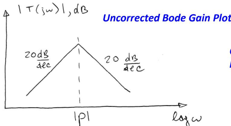
Critically damped case - Resonance is apparent but still not sharp enough.
