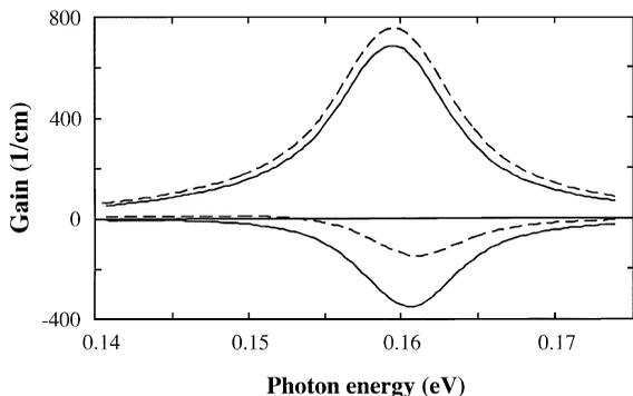
Fig. 4. Gain versus photon energy for quantum-well laser for two phonon models: dashed lines – bulk GaAs LO phonons; solid lines — full spectrum of confined, interface, and half-space phonon modes. The two curves exhibiting positive gain were calculated with an escape time of 0.4 ps and the two curves exhibiting maximum negative gain near 0.16 eV were calculated for an escape time of 0.6 ps.
