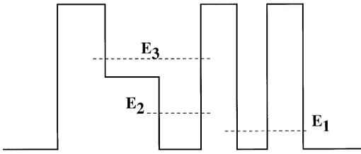
Fig. 1. Step quantum-well laser with  $E_1$  and  $E_2$  separated by the LO-phonon energy.
