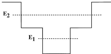
Fig. 2. Single-step quantum-well laser structures.
