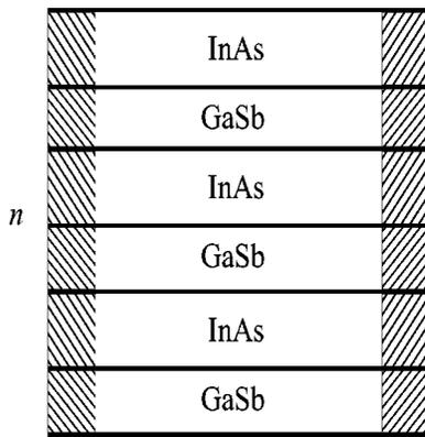
FIG. 1. InAs/GaSb superlattice. The shaded areas show doped regions of the superlattice for the  $n$  and the  $p$  contacts.
