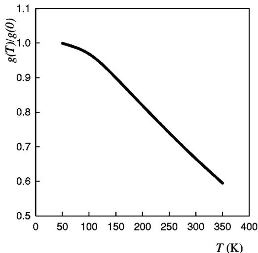
FIG. 4. Temperature dependence of the gain for the carrier concentration in the active region  $10^{12} \text{ cm}^{-2}$ .
