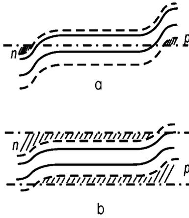
FIG. 3. Band bending and the carrier distribution along the layers of the superlattice. Letters  $n$  and  $p$  show the contacts, solid lines are the bottom of the conduction band and the top of the valence band, the dashed lines are the  $e1$  and  $hh1$  levels, dashed area shows energy regions filled with carriers. (a) Equilibrium, no voltage is applied. Dot-dashed line is the Fermi level. (b) Operating regime. Dot-dashed lines show the quasi-Fermi levels of electrons and holes.
