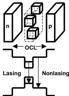
**Figure 2.** Schematic view and energy band diagram of a conventional QD laser.
