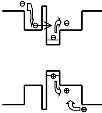
**Figure 6.** Schematic band diagram of tunneling-injection QD lasers reported in [19, 20]. Carriers of one type only (electrons) are tunneling. The tunneling barrier separates the region where electrons are hot from the rest of the structure containing the active layer with QDs. Electrons thermalize before tunneling through the barrier, so that tunneling electrons – to be captured by QDs – are already cold.
