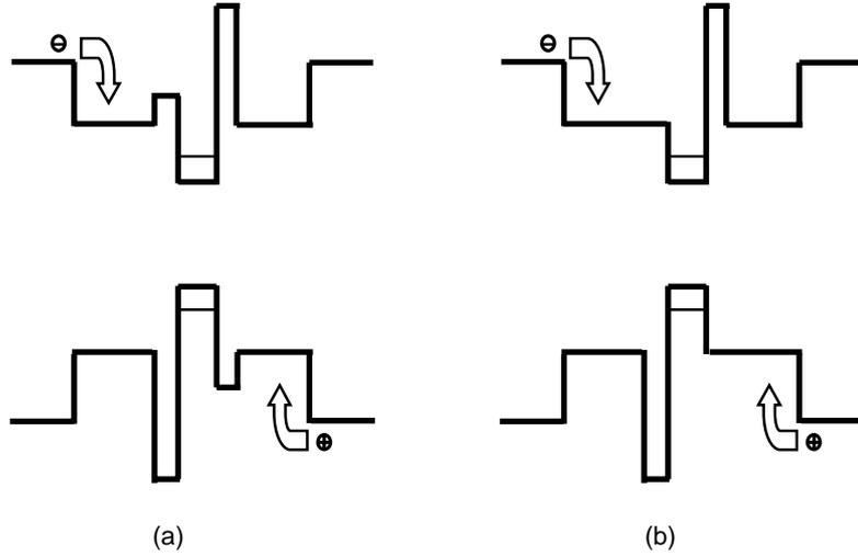
**Figure 7.** Prevention of thermo-activated parasitic recombination in the OCL by band-gap engineering. QDs (shown with energy levels) are clad by heterostructure barrier layers that block only the minority carrier transport.
