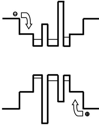
**Figure 5.** Energy band diagram of a tunneling-injection QD laser wherein the tunneling leakage is suppressed by independent variation of the barrier heights for electrons and holes.
