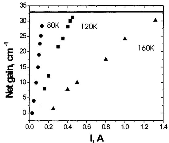
FIG. 2. Dependences of the net gain maxima on current for the sample with 10-W-QWs at three temperatures. Horizontal lines indicate  $\alpha_{\text{tot}}$ .
