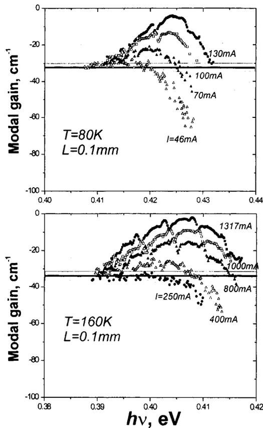
FIG. 1. Spectral dependences of the modal gain for the laser with 10-W-QWs at 80 K (upper panel) and 160 K (lower panel).
