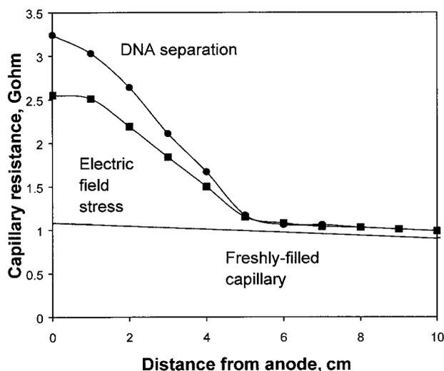
**Figure 2.** Specific resistance plotted as function of distance from the anodic end of the capillary measured by consecutive clipping of 1 cm pieces of the capillary from the anodic end. Experiments were carried out with pure buffer in the anode vials.
