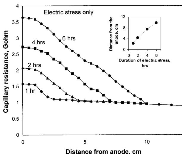
**Figure 3.** Dynamics of the development of the resistive region. The insert shows the rate of the expansion of the resistive region from the anode as a function of time.
