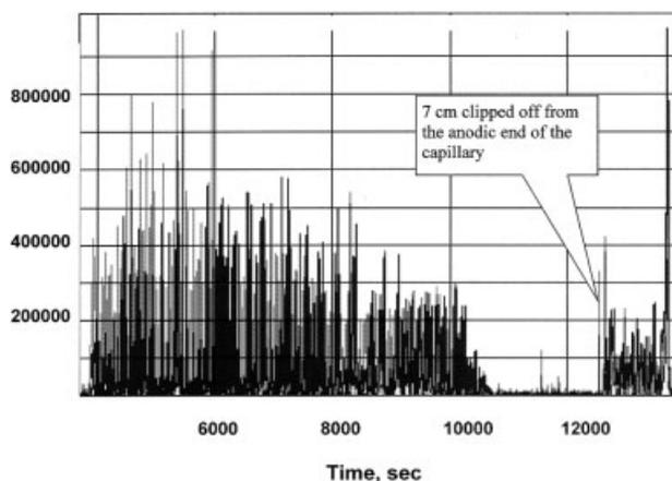
**Figure 5.** Electropherogram of the two-stage separation process. In the first stage, the resistive region  $\sim 6$  cm long was formed at the anode. The motion of the peaks was completely extinguished. Before the second stage, the anodic end of the capillary (7 cm long) was clipped off, and the separation voltage applied again. The peaks resumed their motion.
