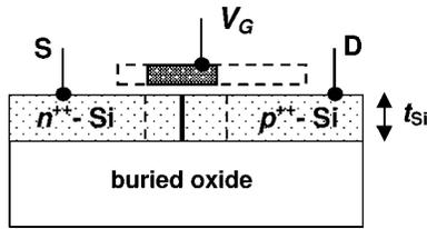
FIG. 1. Schematic layout of a LITT implemented in SOI, bold line marks the  $pn$  junction while the dashed lines indicate the corresponding lateral depletion region. In the ideal LITT, the gate overlaps the depletion region only to minimize capacitance (hatched); in our first fabricated prototypes, the gate overlaps the source and drain regions (dashed).
