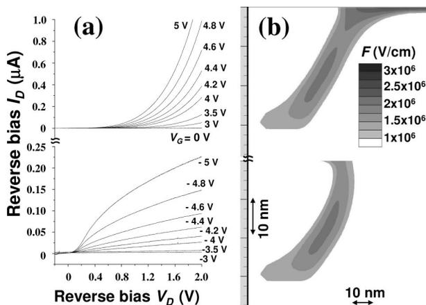
FIG. 2. (a) Reverse-bias  $I_D(V_D, V_G)$  curves for LITT with  $pn$  junction doping of  $6 \times 10^{19}\text{--}10^{20} \text{ cm}^{-3}$  at  $T = 300$  K as a function of  $V_G$  (device parameters: gate length  $L_G = 0.35 \mu\text{m}$ , width  $W = 10 \mu\text{m}$ , Si film thickness  $t_{\text{Si}} \sim 40$  nm, gate oxide  $\sim 5$  nm); (b) Simulations of the spatial variation of  $F$  in the device for  $V_G = 2$  V (upper) and  $V_G = -2$  V (lower), both at  $V_D = -1$  V.
