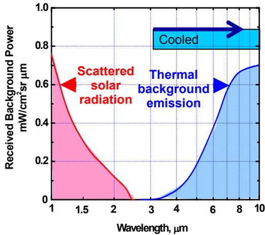
**Fig. 2.** Spectral dependence of the background optical power received by a terrestrial detector.
