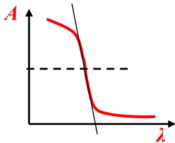
**Fig. 4.** Spectral response of a detector effecting direct optical frequency discrimination.
