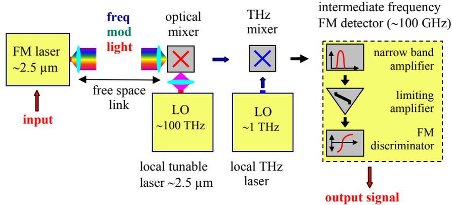
**Fig. 5.** Schematic diagram of a multi-channel free-space communication link based on optical frequency modulation and heterodyne detection
