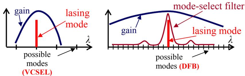
Fig. 3. Tunable single-mode lasers, vertical-cavity surface-emitting lasers (VCSEL) and distributed-feedback lasers (DFB).
