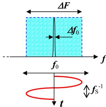
**Fig. 1.** Nomenclature of frequencies involved in a FM communication link.
