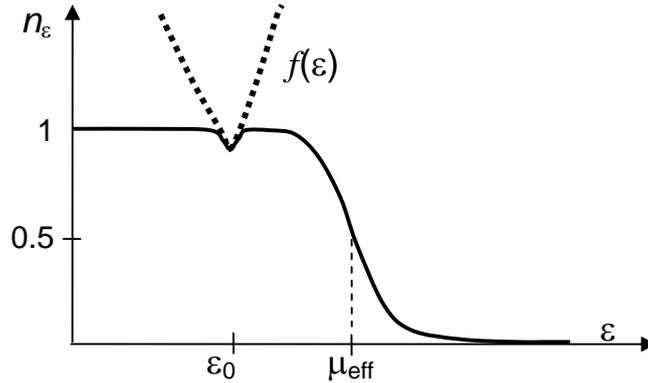
**Figure 2.** Schematic representation of the electron energy distribution  $n_\varepsilon$  and the function  $f(\varepsilon) = \sigma_\omega / \gamma_\varepsilon$ . These functions coincide in region  $\Gamma$ .
