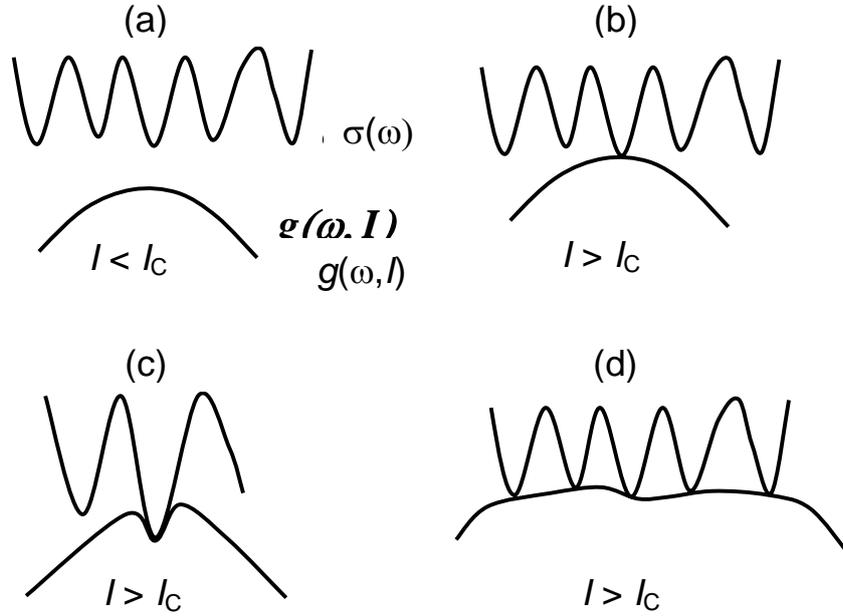
**Figure 1.** Relative configuration of the spectral curves corresponding to the material gain  $g(\omega, I)$  and the loss  $l(\omega)$  of the electromagnetic field intensity at the cavity mirrors below (a) and above (c-d) the threshold  $I_c$ .
