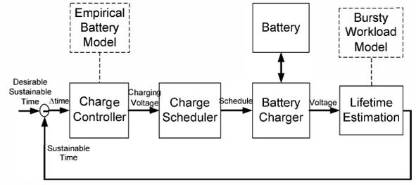
Fig. 4: Battery Charge Control Loop
