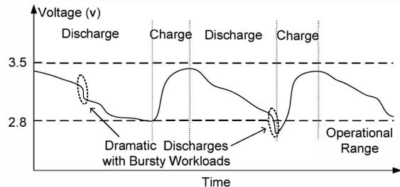
Fig. 1: Battery Charge with Bursty Load
