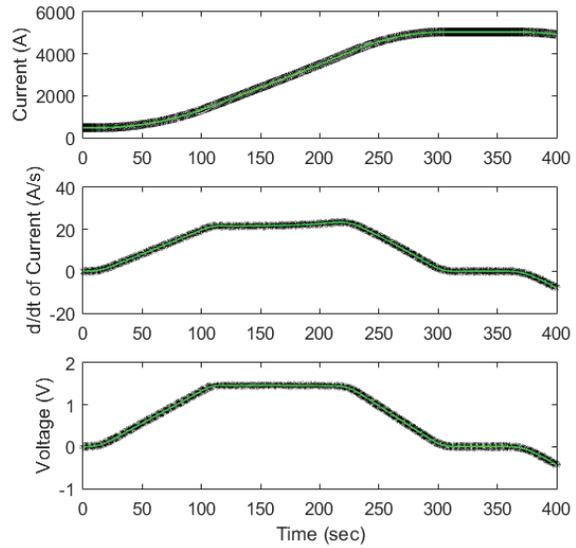
Figure 3: Raw and filtered I, dI/dt and V
