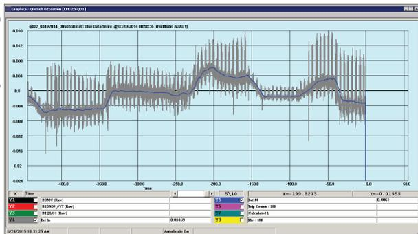
Figure 7: Field testing, quench trigger signal
