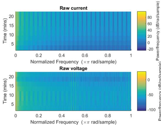
Figure 2: Spectrograms of voltage and current signals
