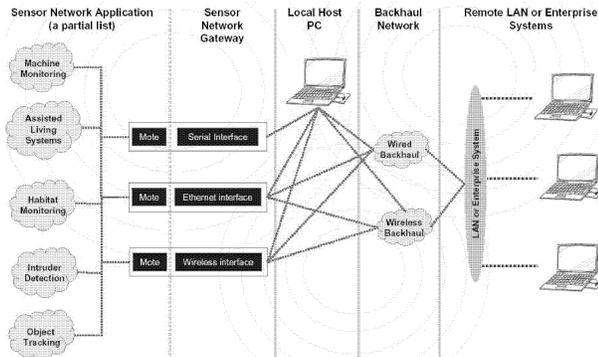
Fig. 2. Sensor Network Architecture
