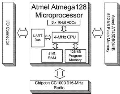
Fig. 4. Schematic for the hardware configuration
