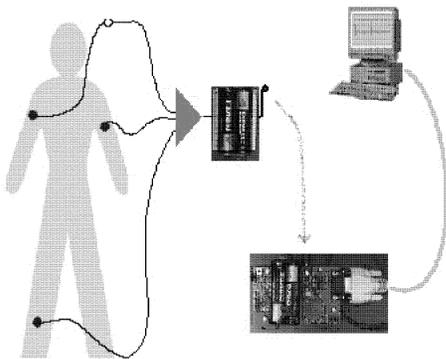
Fig. 5. Bio Potential Imager's Prototype
