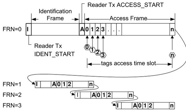
**Figure 1. Frame structure of the proposed collision resolution protocol.**
