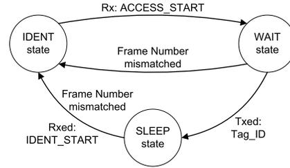
**Figure 2. Tag state machine of the proposed collision resolution protocol.**
