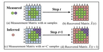
Fig. 6. The illustration of the sampling stopping condition. Fig.6(a) and Fig.6(c) are the measurement matrices at step t and step t + 1, respectively. Fig.6(b) and Fig.6(d) are the recovered matrices at step t and step t + 1, respectively. If the recovered matrices satisfy  $\hat{X}(t) \stackrel{\Delta}{=} \hat{X}(t+1)$ , stop sampling at step t+1; else add more samples in the next sampling step t+2.
