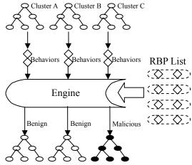
Figure 3. Malware detection engine. It monitors raw behaviors and marks a cluster as malicious if the cluster exhibits any predefined RBP.
