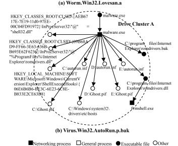
Figure 4. Dependency graph examples of four tested malware samples
