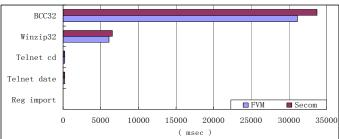
Figure 7. Applications' overall performance. Secom only imposes 0.8%~8.3% additional overhead on independent applications.
