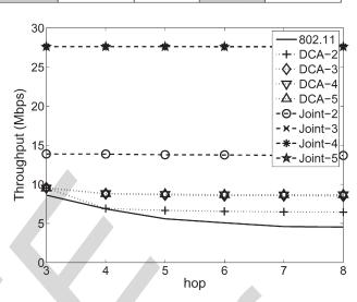
Fig. 6. Throughput in the chain topology.
