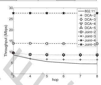
Fig. 6. Throughput in the chain topology.
