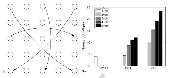
Fig. 7. Performance for the grid topology. (a) Topology. (b) Throughput.
