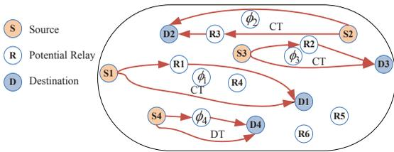
Fig. 3. Adding virtual relay nodes for uniformed relay assignment.
