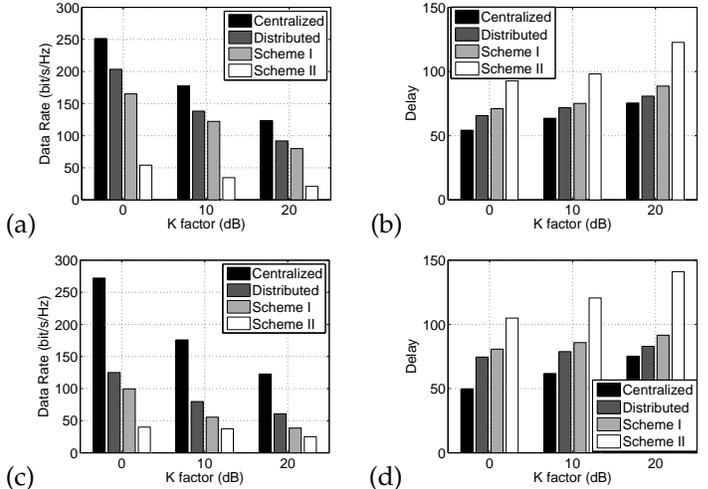
Fig. 6. Impact of LOS component and variance of antenna array size. With variance = 1: (a) data rate; (b) delay. With variance = 2: (c) data rate; (d) delay.
