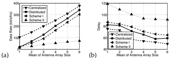
Fig. 3. Impact of mean of antenna array size: (a) data rate; (b) delay.
