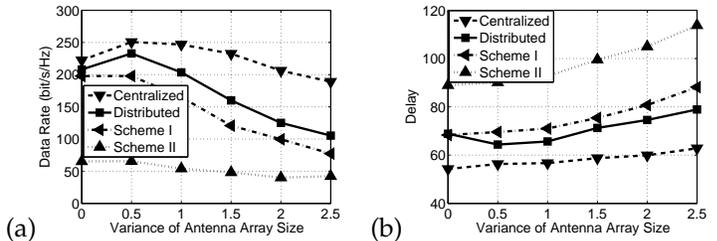
Fig. 4. Impact of variance of antenna array size: (a) data rate; (b) delay.
