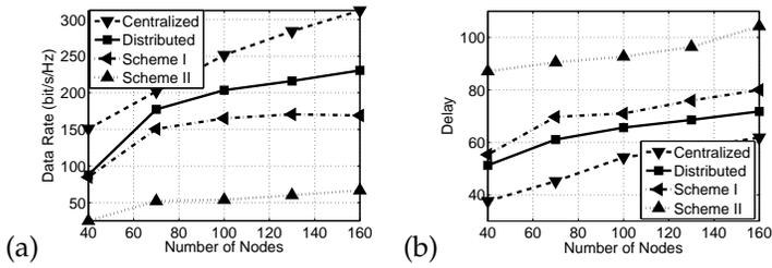
Fig. 7. Impact of node density: (a) data rate; (b) delay.
