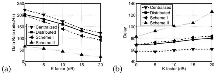
Fig. 5. Impact of LOS component: (a) data rate; (b) delay.
