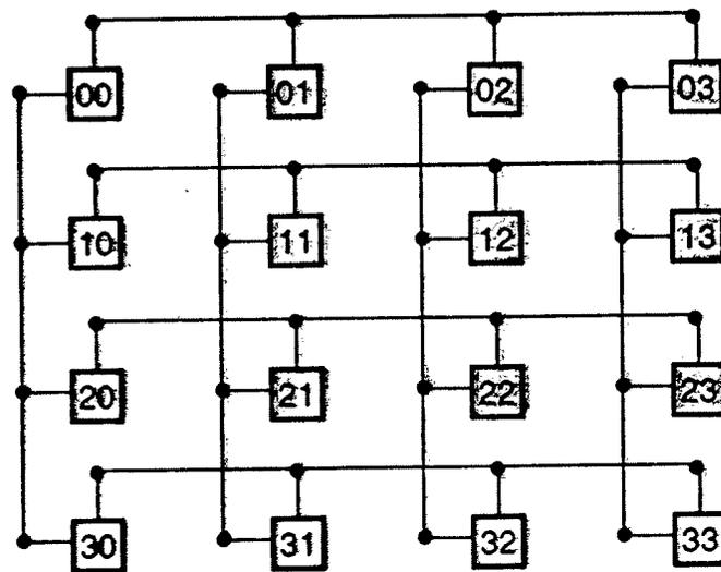
**Figure 1.16** A  $4 \times 4$  mesh of processing elements (PEs) with broadcast bus for each row and on each column. (Courtesy of Prasanna Kumar and Rajendra; reprinted from *Journal of Parallel and Distributed Computing*, April 1991)
