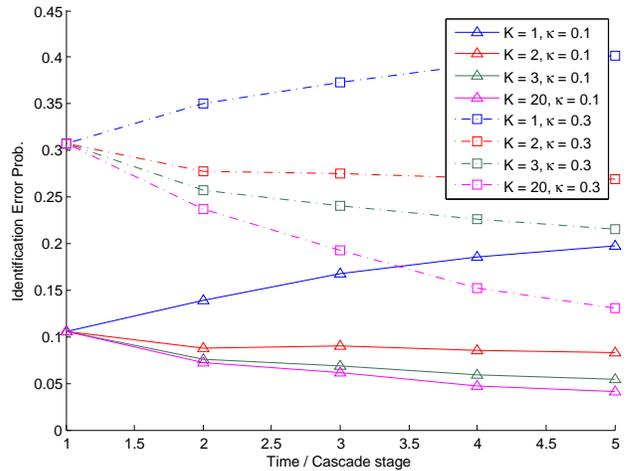
Fig. 3. Error probability for identifying the outage pattern at different cascade stages in the IEEE 14-bus system.
