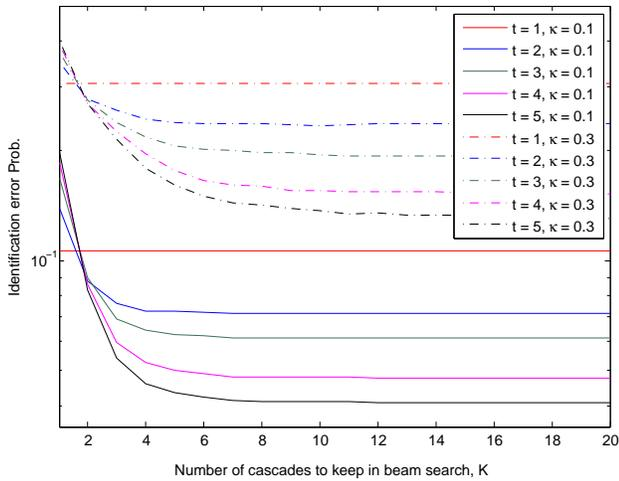
Fig. 5. Error probability for identifying the outage pattern with different numbers of cascades retained in beam search in the IEEE 14-bus system.
