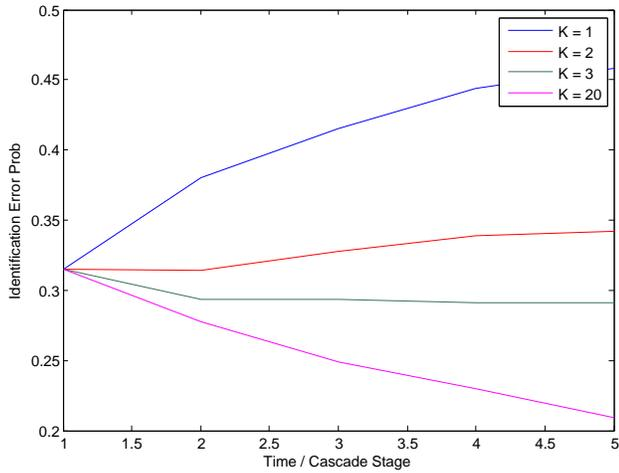
Fig. 4. Error probability for identifying the outage pattern at different cascade stages in the IEEE 57-bus system.
