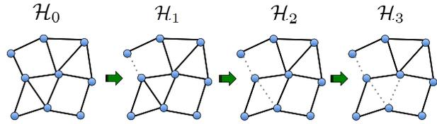
Fig. 1. The development of cascading failures over time. The solid and dashed lines denote the connected and disconnected transmission lines, respectively.
