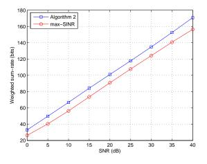
Fig. 3. Performance of Algorithm 2 in  $(6 \times 6, 2)^5$  interference channels:  $w_1 = w_2 = 0.1, w_3 = w_4 = 1, w_5 = 10.$
