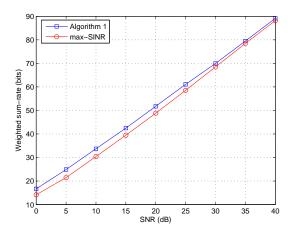
Fig. 2. Performance of Algorithm 1 in  $(3 \times 3, 1)^5$  interference channels:  $w_1 = w_2 = 0.1, w_3 = w_4 = 1, w_5 = 10.$
