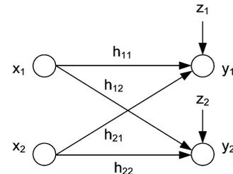
Fig. 1. Two-user Gaussian interference channel.
