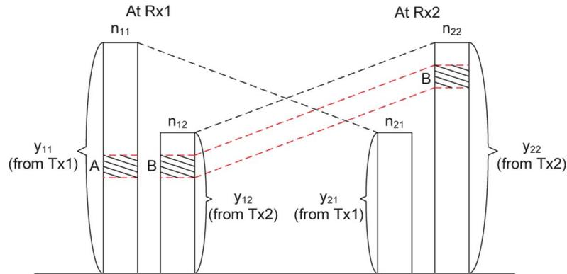
Fig. 4. Two-user deterministic interference channel. Levels A and B interfere at the first receiver, and cannot be fully active simultaneously.
