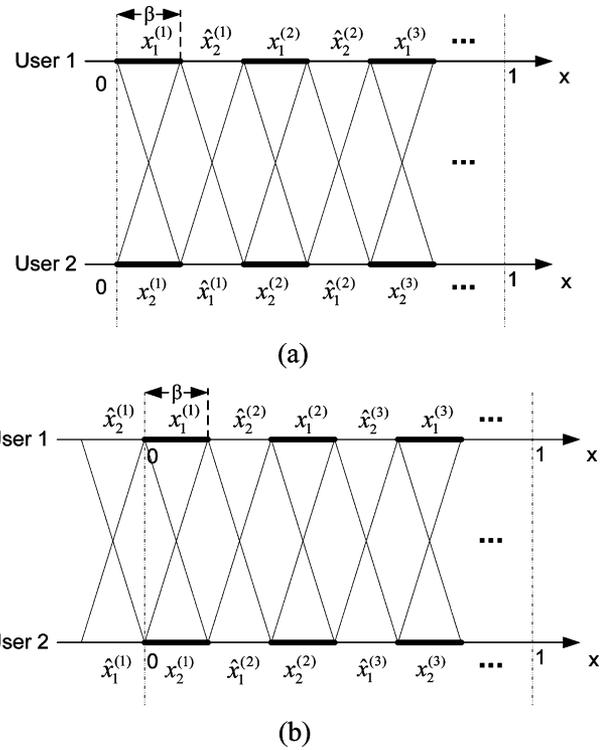
Fig. 12. The optimal schemes in the symmetric deterministic interference channel. (a) Weak interference channel. (b) Strong interference channel.
